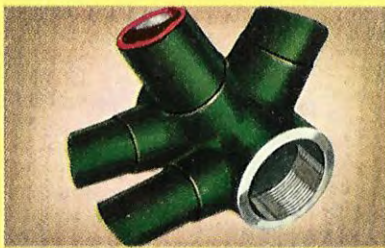
RALEIGH SEAMLESS BOTTOM BRACKET. A circular flat disc of finest quality steel is scientifically manipulated by powerful presses, involving over 30 operations with frequent normalizing treatment to remove stresses set up, into an immensely strong bottom bracket without a join of any description.
