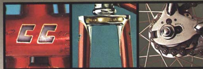
1 - Carlton initial cutout in bottom bracket shell
