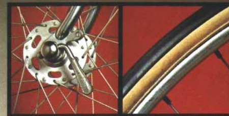
1 - Quick release wide flange alloy hubs
