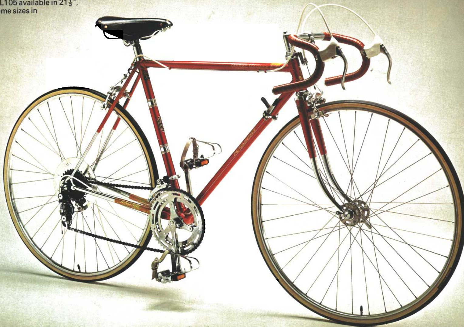
2 - Alloy hollow section sprint rims with tubular tires
