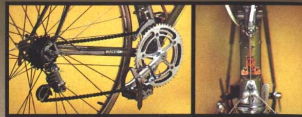
1—Campagnolo chainwheel set, pedals, hubs, and gears
