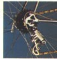
New Campagnolo Super Nuovo Record featuring titanium parts for minimum weight.
