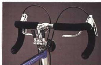
Cushioned handlebar grips, brake extension levers, and stem shifters are standard features.
