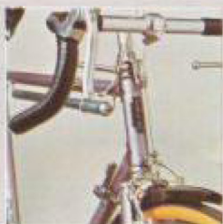
Alloy centre-pull brakes with GT extension levers. Ball-bearing steel quill pedals. The Circuit is also available in Polychromatic Violet.
