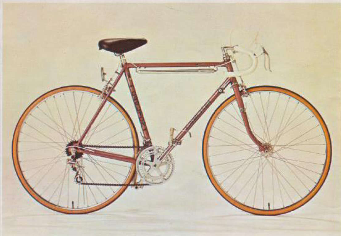
Reynolds '531' main tubes. Alloy cotterless chainset with integral chainguard ring for Giro.
