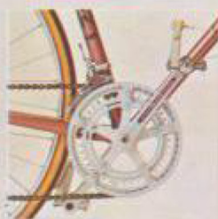
Reynolds '531' main tubes. Alloy cotterless chainset with integral chainguard ring for Giro.
