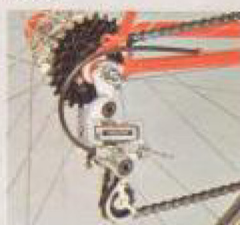
Alloy 10-speed gear mechanism with ratchet levers.
