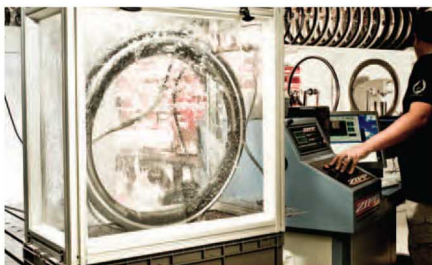
Inflating with water instead of air saves rims and eardrums when testing for maximum tire pressure.
