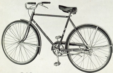
Men's Tourist equipped with Schwinn Rear Expander Brake
