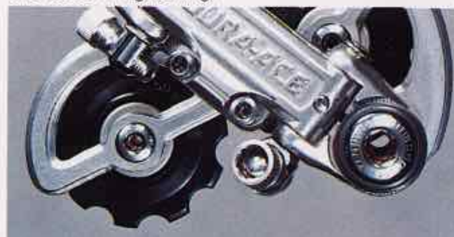
All the bolts are 3mm. or 6mm. hexagonal bolts.
