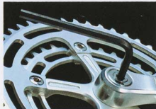
Hexagon wrench key (8 mm.) with Shimano 600EX Front Chainwheel (Model GC-400)
