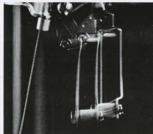
Parallel movement of the conventional pantograph mechanism.
