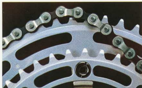
Gear shift on W-cut Teeth
