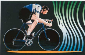
50km/h Air resistance for rider and bicycle is 3.61kg (7.96 lbs.) (About 31 mph)
