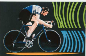
50km/h Measuring bicycle and rider separately (About 31 mph) Human Body Air Resistance 2.39kg (5.27 lbs.) Bicycle Air Resistance 1.22kg (2.69 lbs.)
