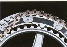
The Chain on Front Chainwheel with aligned large and small gears.
