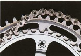
The Chain, on Front Chainwheel without aligned large and small gears, slips on the teeth.
