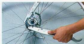
When removing sprockets, as seen in photograph, use the double wrap sprocket turning chain for easier operation.
