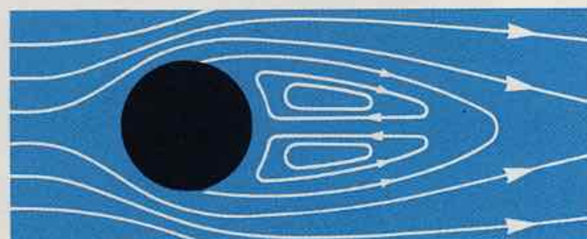
Wind Stream which is directed toward a cylindrical object disturbs air flow.
