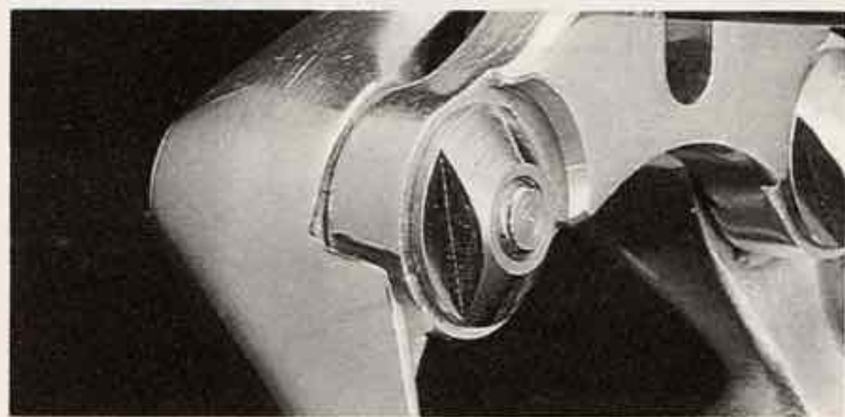
Sealed Mechanism preventing mud, water and unwanted objects from entering for smooth braking at all times.
