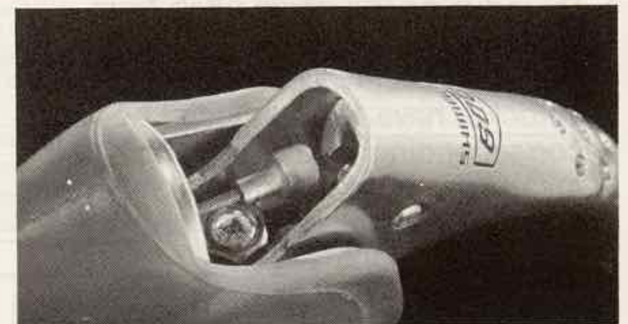
One-step cable attachment mechanism (Shimano-600EX Brake Lever)
