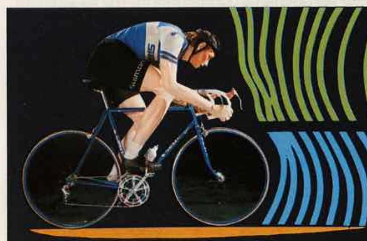
50km/h Measuring bicycle and rider separately (About 31 mph) Human Body Air Resistance 2.39kg (5.27 lbs.) Bicycle Air Resistance 1.22kg (2.69 lbs.)
