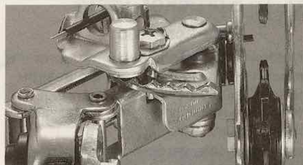
Positive Indexing Mechanism on Positron-II Rear Derailleur
