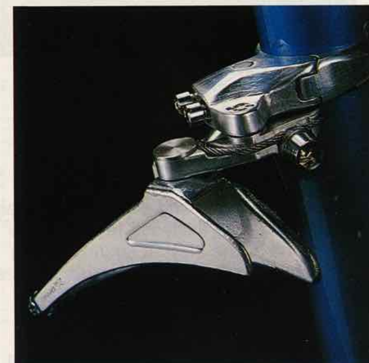
Front Derailleur Cable End Attachment used on Dura-Ace AX, Shimano 600 AX and Adamas AX
