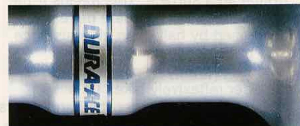
Dura-Ace AX Front Hub which has buff almite finish.
