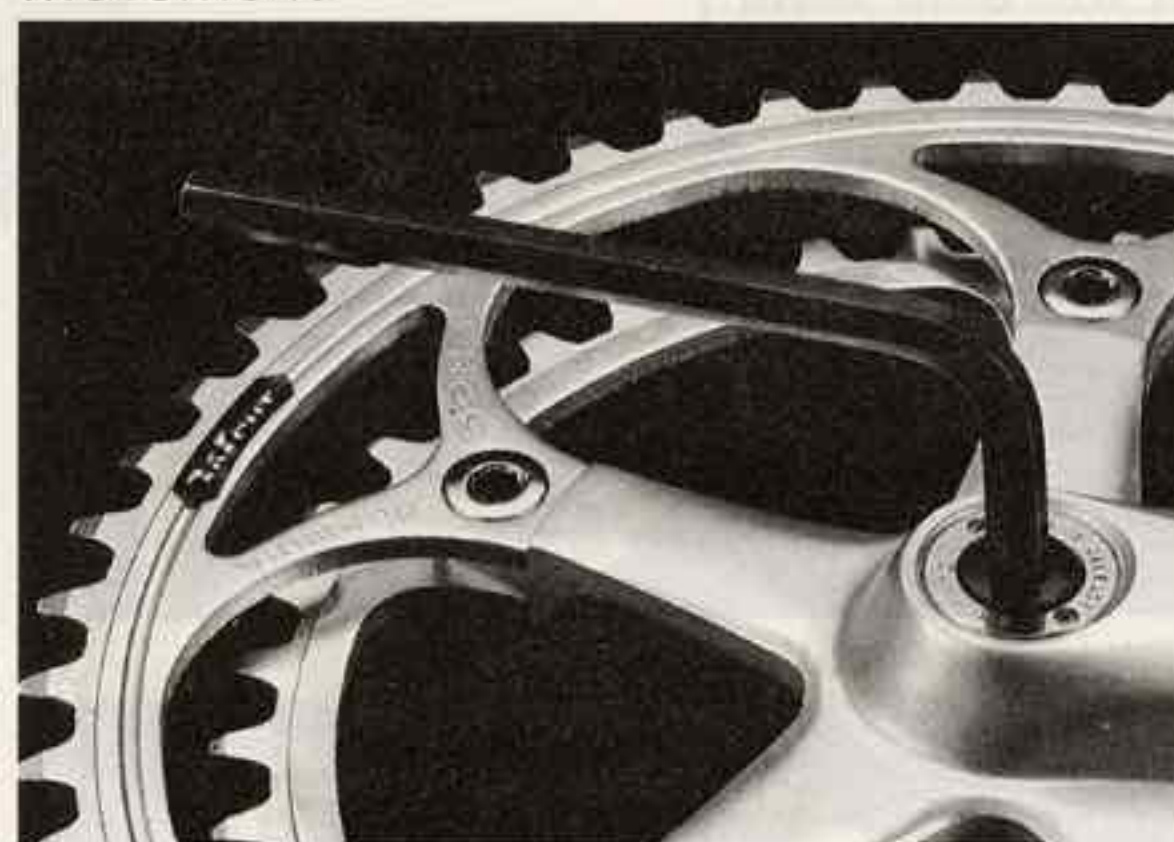
Hexagon wrench key (6 mm.) with Dura-Ace AX Front Chainwheel.
