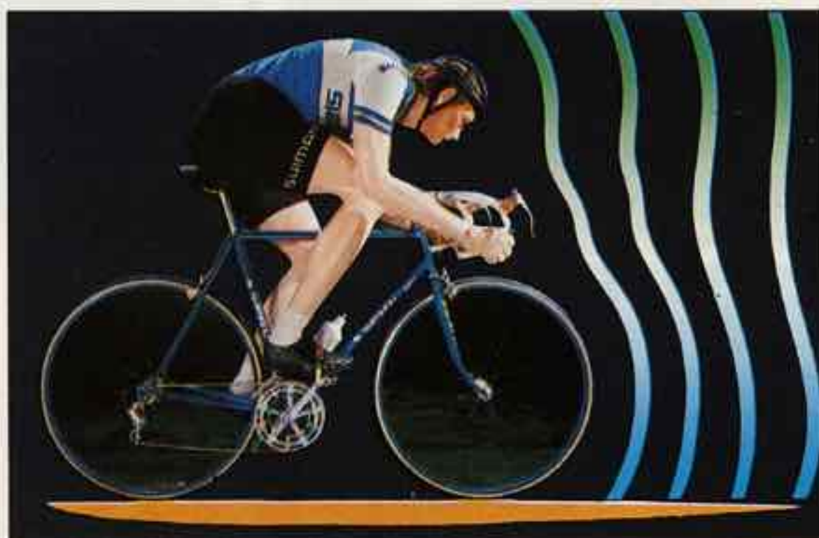
10km/h Air resistance for rider and bicycle is 0.14kg (0.31 lbs.) (About 6 mph)
