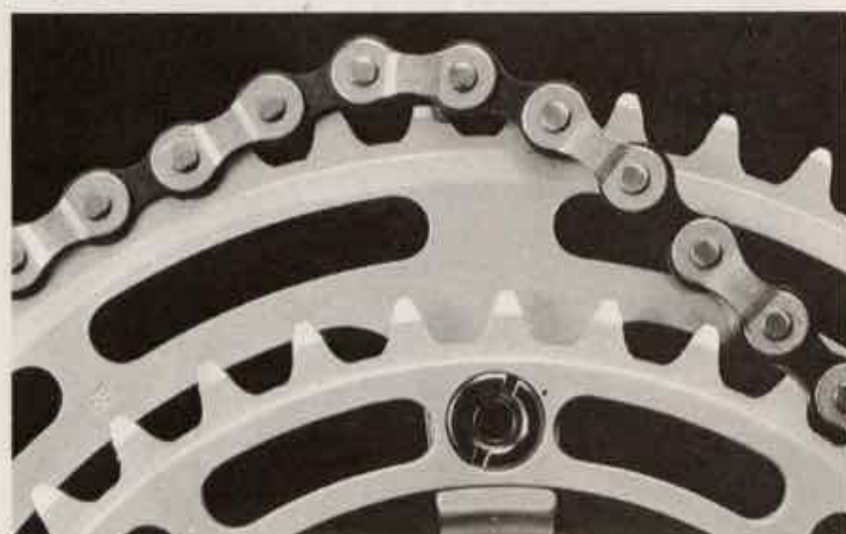
Gear shift on W-cut Teeth
