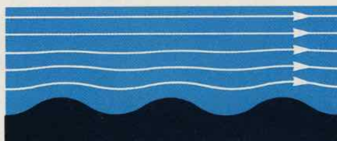
Air disturbance resulting from friction resistance.
