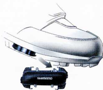
Step in to engage the SPD binding.
