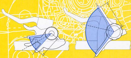
New EZ-Fire lever reduces the front derailleur shifting stroke by over 50%.
