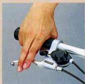
EZ-Fire Plus positions the shift levers so they can be more easily used with fingers resting on the brake lever.
