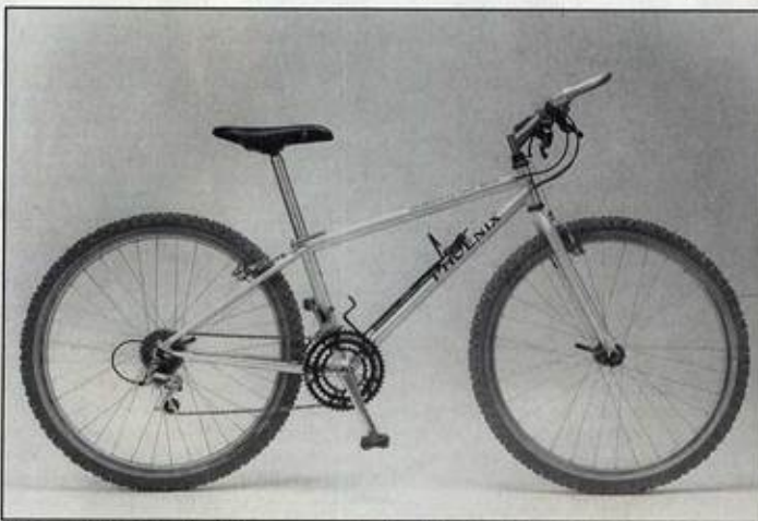
The radically sloping top tube on our smaller test bike created a good amount of standover height for our smaller test riders. Fairly standard angles with a longish fork trail create a more stable than aggressive bike for most trail riding situations.
