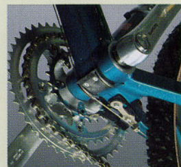
Klein's Chain Control Device™ keeps the chain from sucking between the chainring and chainstay by sweeping it clean and avoiding chain suck.
