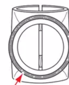
Milled = weakened by gaps
