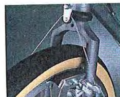
Dia Compe cantilever brakes with motorcycle-type levers.
