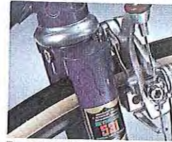
Reynolds 531 fork blades and an investment-cast crown.
