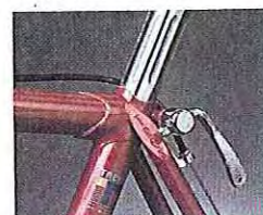
The quick-release seat cluster lets you easily adjust saddle height.
