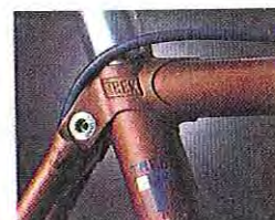
Reynolds 753 tubes joined by Trek's unique cast seat lug.
