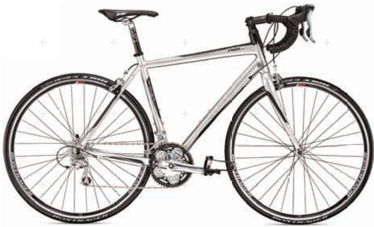
PILOT 2.0™ // FRAME Alpha Black Aluminum // FORK Bontrager Satellite Plus, carbon // WHEELS Alloy Hubs; Bontrager Approved Alloy Rims CRANK FSA Vero 50/39/30 // REAR DERAILLEUR Shimano Tiagra // COLOR Bright Silver / Metallic Black
