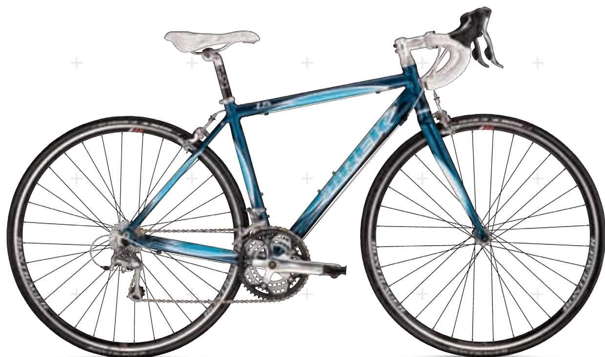
1.5 WSD™ // FRAME Alpha White Aluminum // FORK Bontrager Approved, Carbon // WHEELS Alloy Hubs; Bontrager Approved Alloy Rims CRANK FSA Vero 50/39/30 // REAR DERAILLEUR Shimano Tiagra // COLOR Plumage
