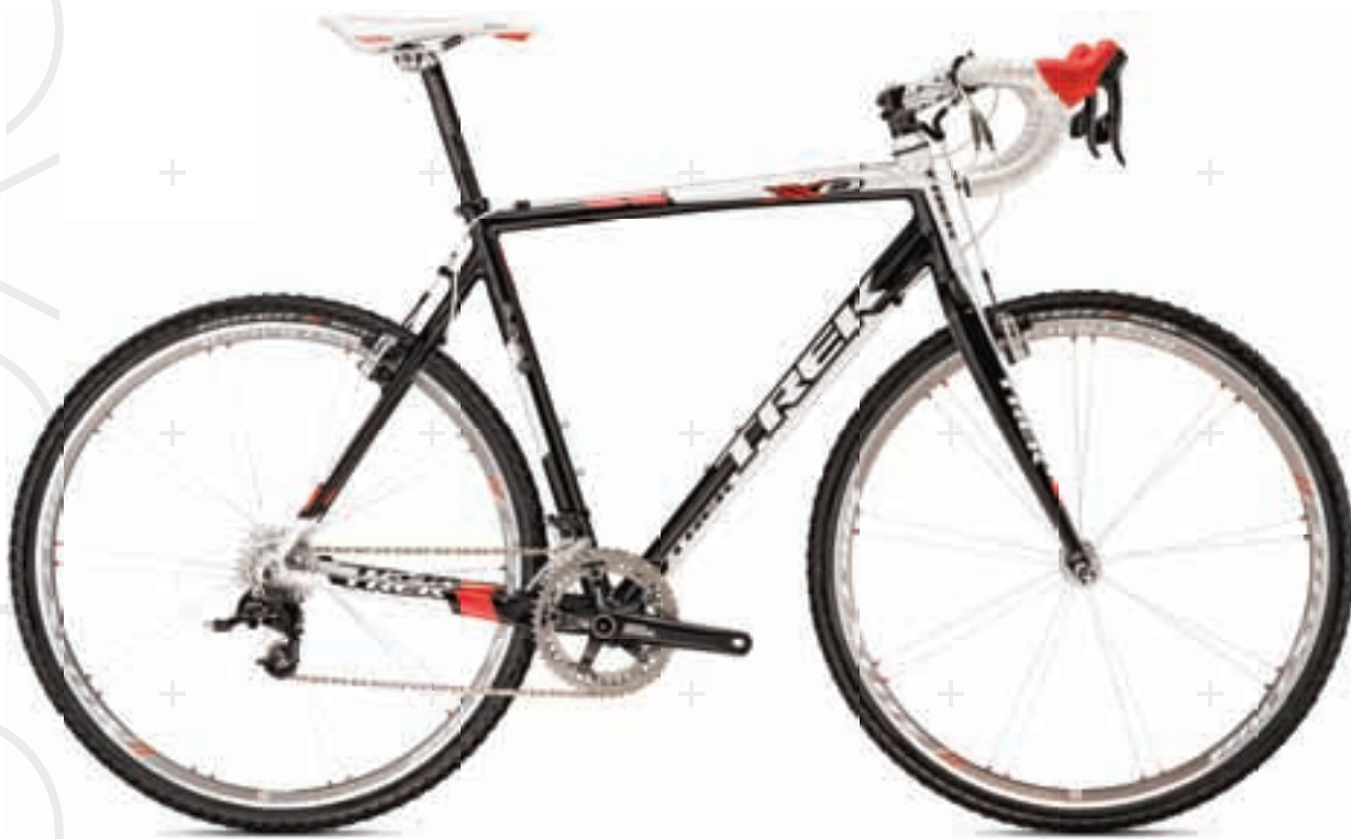
XO2™ // FRAME Alpha Black Aluminum // FORK Bontrager Satellite Plus, carbon legs // WHEELS Bontrager Race X Lite CRANK SRAM Rival OCT CX 46/38 // REAR DERAILLEUR SRAM Rival // COLOR Gloss White / Gloss Black / Red
