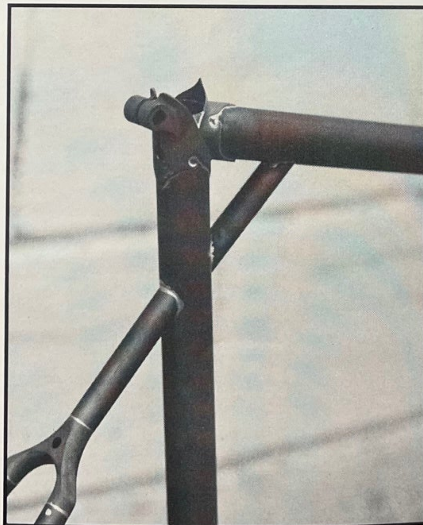
top: Unique, hand-cut and polished stainless steel seat cluster. bottom: Clean workmanship is evident on this aerodynamic seat cluster.
