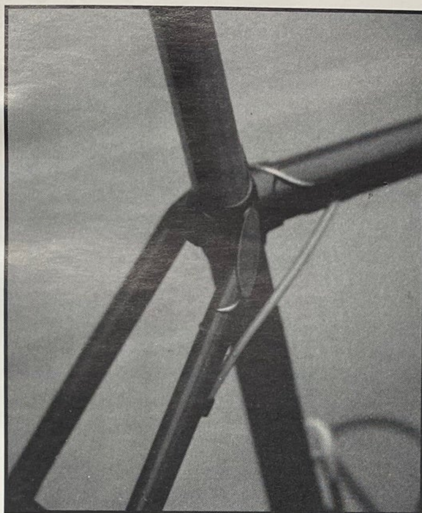
top: Unique, hand-cut and polished stainless steel seat cluster. bottom: Clean workmanship is evident on this aerodynamic seat cluster.
