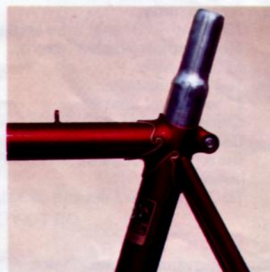
Superlight style seat stays and allen key bolt seat lug.
