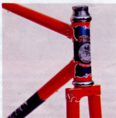
Nervex lugs and Hand cut King of Mercia crown.
