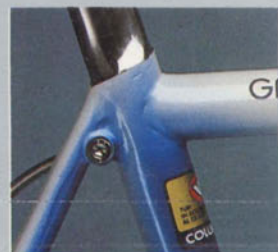
Brazed-on frame integrated seat post clamp
