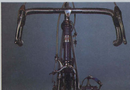
CAMPAGNOLO TRIOMPHE brakes with forged alloy levers.
