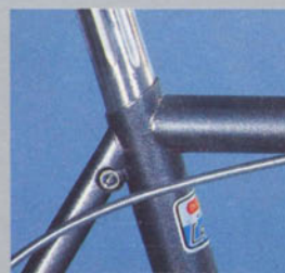
Brazed-on frame integrated seat post clamp
