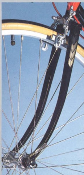
Sloping crown fork and quick release
