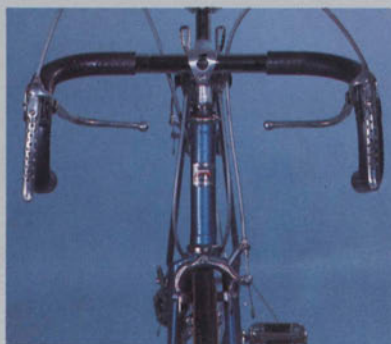
MOTOBECANE sleeve and dual control levers
