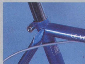
Brazed-on seat post clamp
