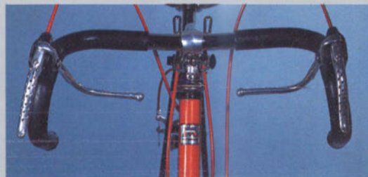
WEINMANN side pull with AUTO-LUBE cables
